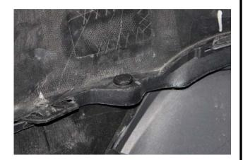
9. Next remove the two screws that attach the large plastic tabs in the center of the diffuser.
