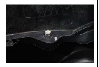
13. In the two center holes (formerly occupied by the push-type clips), use the provided bolts and jam nuts to affix the diffuser to the rear bumper cover.
