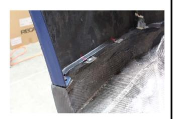
12. Once fitted, attach the provided speed nuts [U-Clips] to each of the tabs along the back edge of the diffuser (15 total) and use the included screws to pass through the OEM tabs and into the speed nuts (holes will need to be drilled in each tab prior to fitting).
