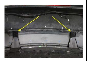
11. Next, carefully fit the Unplugged Performance [U.P.] Rear Under Spoiler to the rear bumper cover, slipping the tabs into the slots in the bumper cover (15 tabs & slots).
